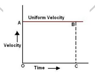
• The magnitude of displacement or distance travelled by the body is equal to the area enclosed by the velocity-time graph and time axis.
