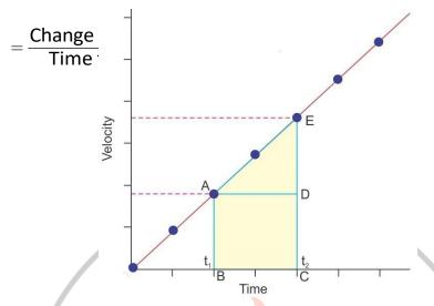
• The slope of the velocity-time graph represents the acceleration of the body.
